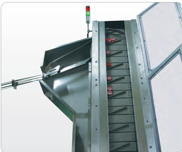
Feeding System (Cap feeding and sorting section)
