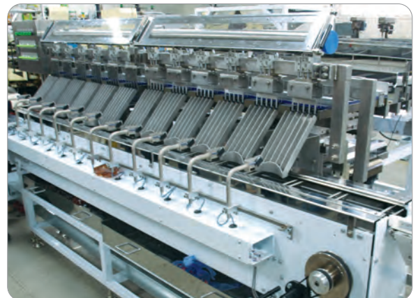
Choco Ball Supply Device (Multi-lanes supply system) (30 lanes × 2 sets)
